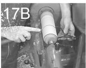
17. (A) Make a jam chuck and mount assembled mill between centers. (B) Using calipers part down to establish the highs and lows of your curves from your template.
