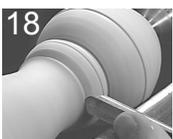
18. Cut shape of mill following template design. Sand to 220 then establish any V-cuts and sand through 1200.
